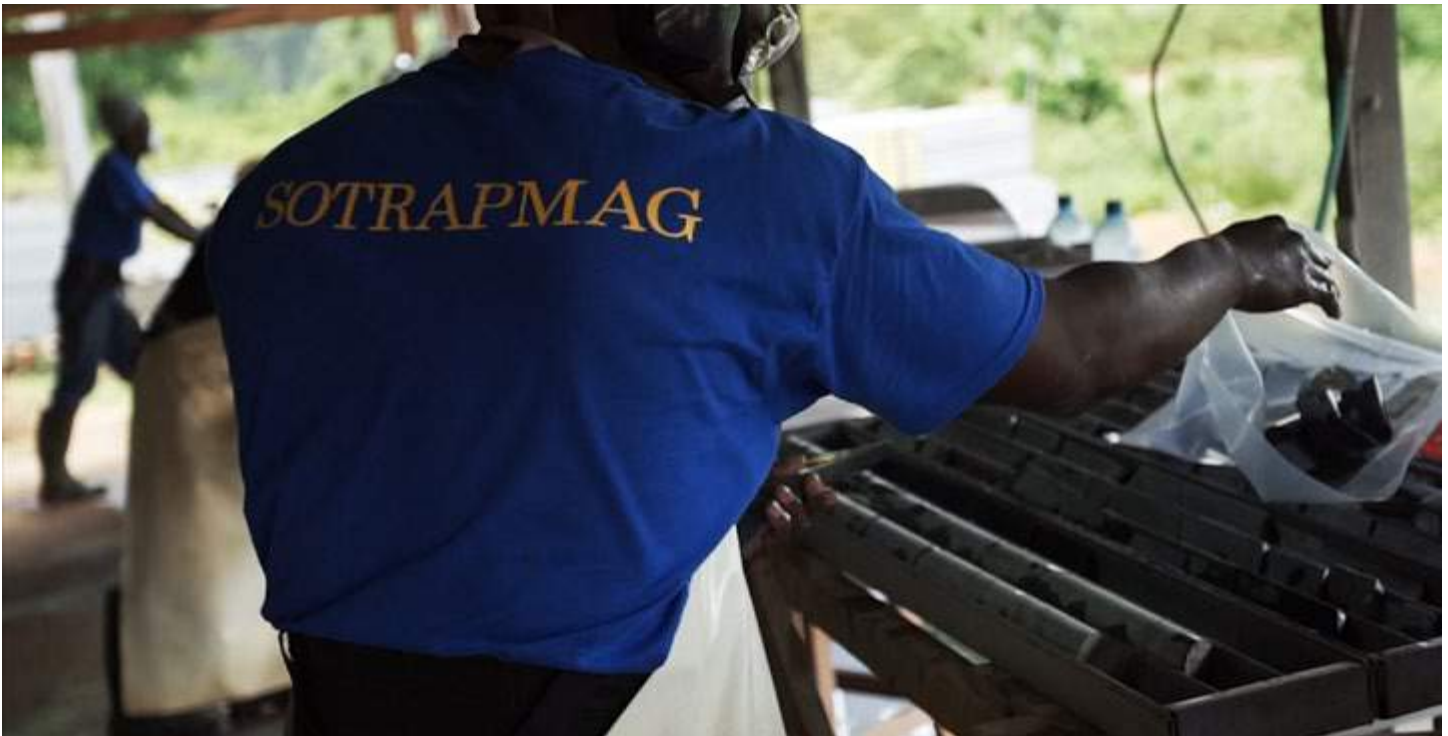
Photo: Preparing core for assaying - Camp Citron, Paul Isnard gold Project, French Guiana.
